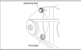
Fig. 34 Adjust Belt Tension
